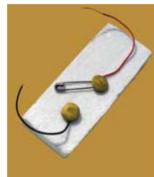
Figure 41.1 A simple switch
