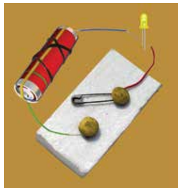
Figure 41.2 An electric circuit with a switch
